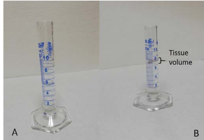
Figure3. Application of Archimedes' principle to measure volume. A) Graduated cylinder filled with water, B) Volume of the tissue calculated by the increase in total volume.
